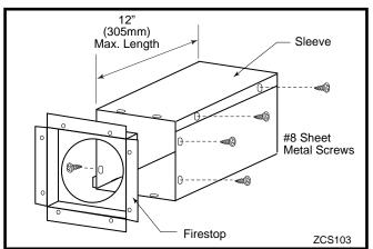
Fig. 25 Assemble the wall sleeve and firestop.
